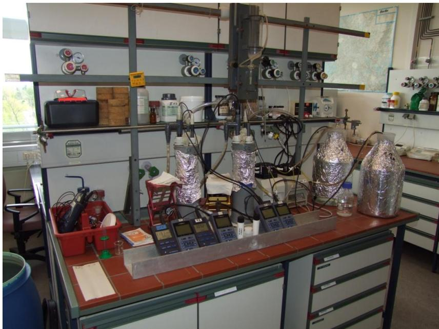
**Figure 3-1: Columns of the leaching experiment in the laboratory**
